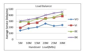
Figure 7. Average delay variation of four access categories (Load Balance).
