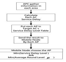
Figure 4. Mobile Node Handoff Architecture.
