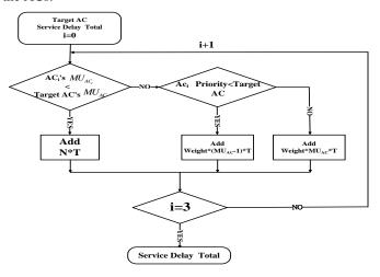
Figure 2. Flowchart for the computation of service delay.
